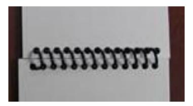
The third pad to the right with the black binding illustrates a true spiral binding. This binding type was found to snag on the double j-channels and become unbound quickly rendering the pad unusable. SCEL does NOT wish to procure this type of spiral binding.
